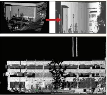
Figure 6: 2D range image of the point cloud
